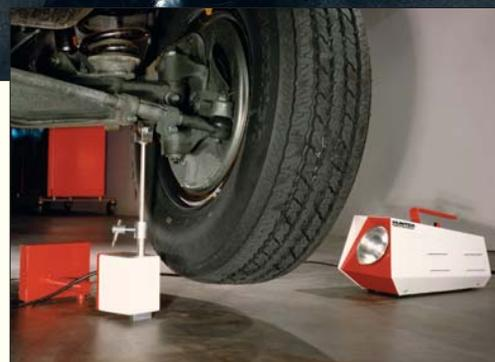
**The Strobe Balancing System balances the entire wheel assembly, helping technicians detect a wide range of imbalance conditions.**
