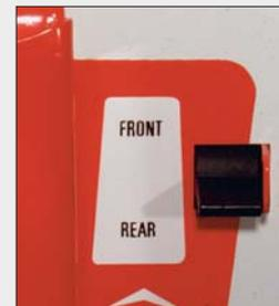
*Front/Rear switch compensates for phase switch between drive and non-drive wheels.*
