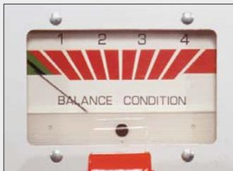
*The amount of weight required for an accurate balance is shown on the balance indicator.*
